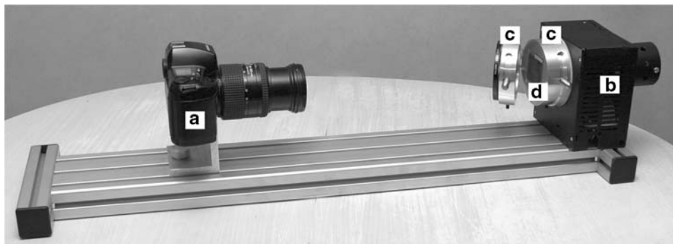
Fig. 1 The photographic set up; (a) digital camera, (b) illuminator equipment with a halogen light, (c) nicoles and (d) a thin-section/sample holder
